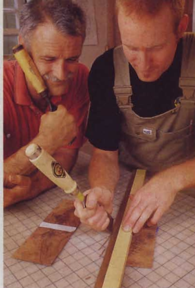
The background of a marquetry pattern can be "knife-cut" with a sharp chisel, as apprentice Thilo Roemer does here while Paul looks on.
